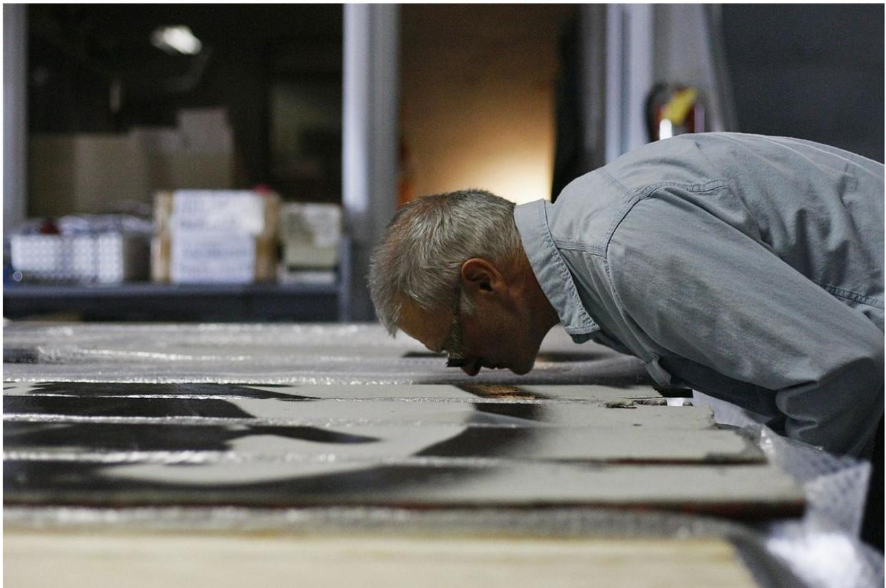
Paul Schurch, Master Woodworker, inspects under magnification details of the mural's redwood slats while planning the mounting system to a honeycomb panel.
